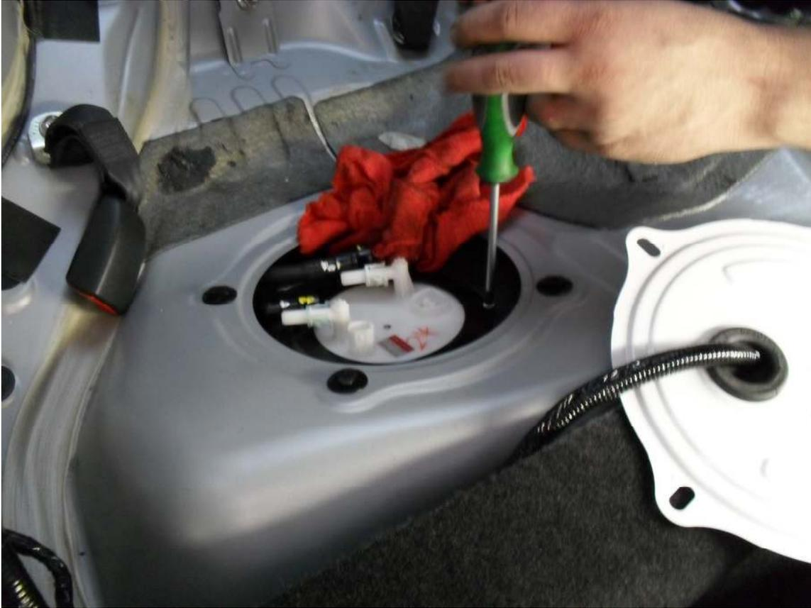
6. Place rags around the area to absorb any leaking fuel. Lift the bulk head away. Once clear, press the lock tab located beneath the tall end of the fuel pump housing. Slide the housing backwards and lift it free from the fuel tank.
