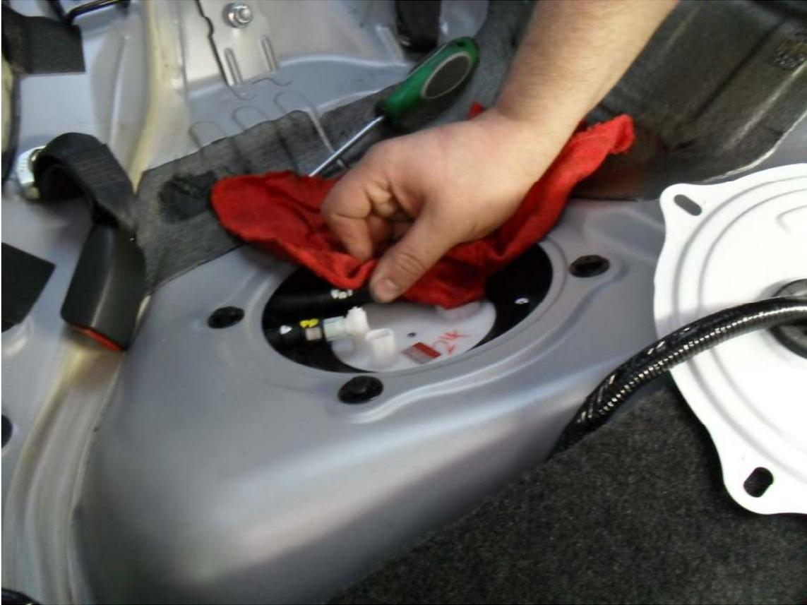
5. Remove the six 8mm bolts. You can also use a Phillips screw driver to remove them. Lift the ring upwards.
