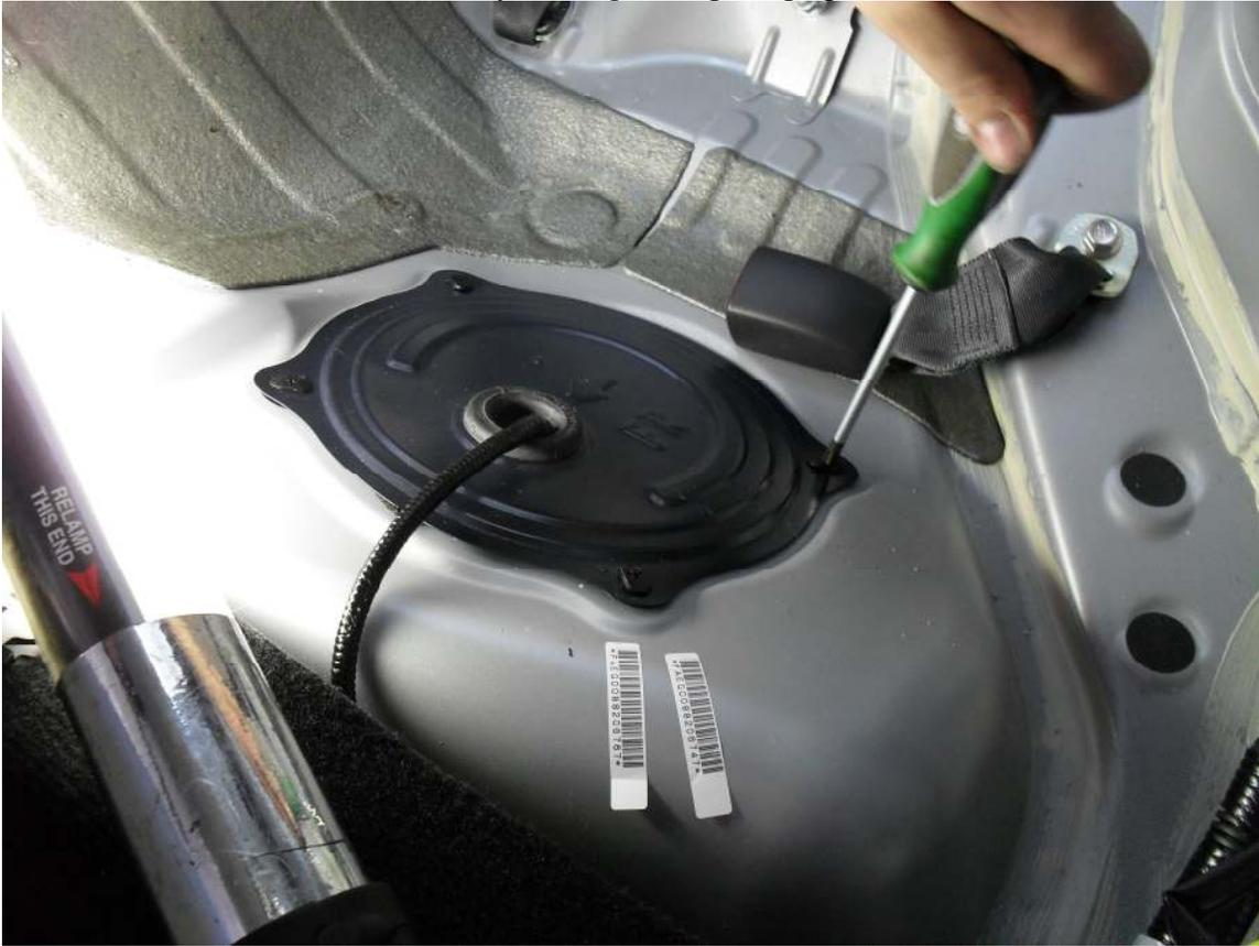
3. Unplug the fuel sending unit connector and fuel pump connectors from the pump bulk head by pressing the lock tab and pulling upwards on the connector.
