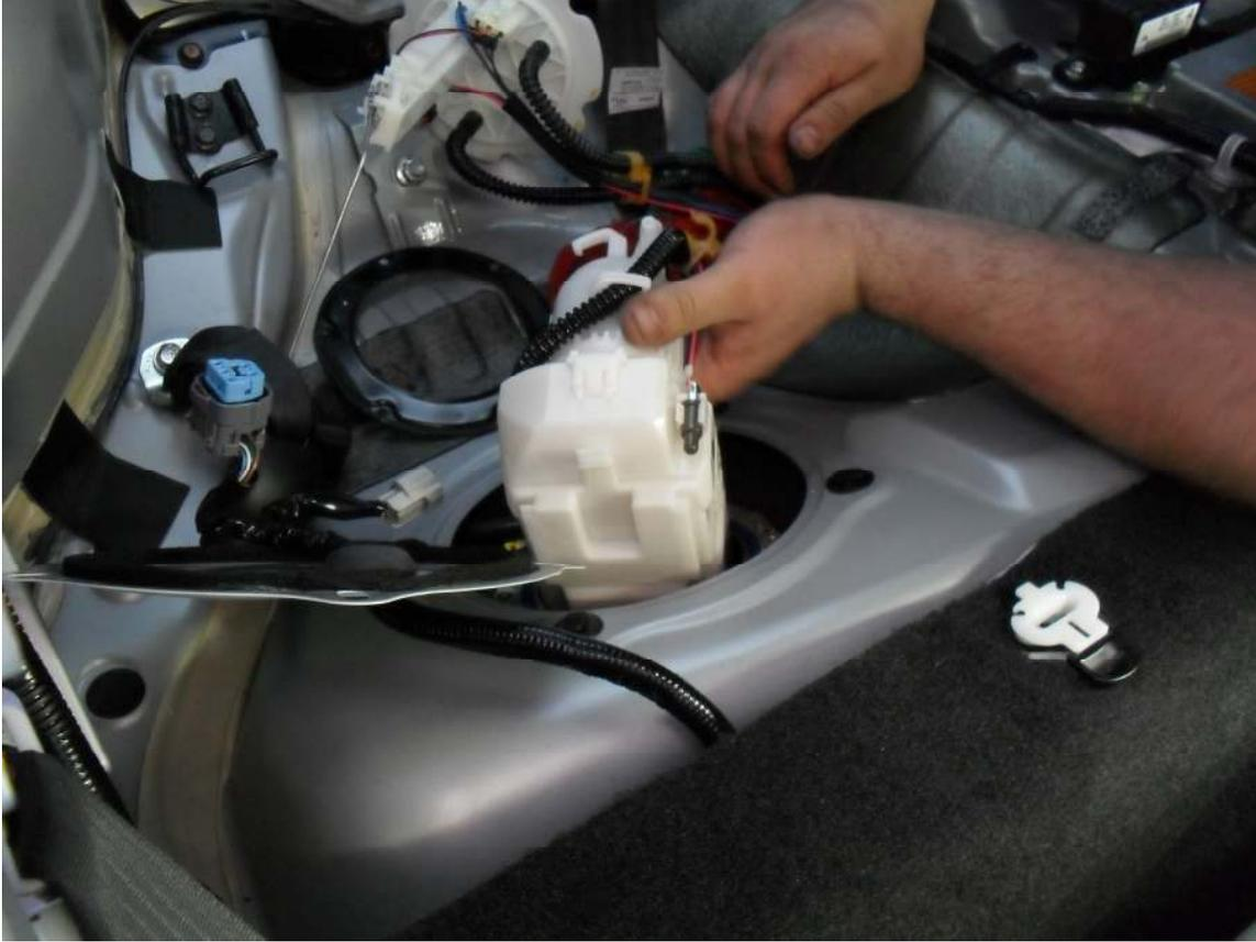
7. Lift the pump housing free and disconnect the three fuel lines from the pump housing's body.
